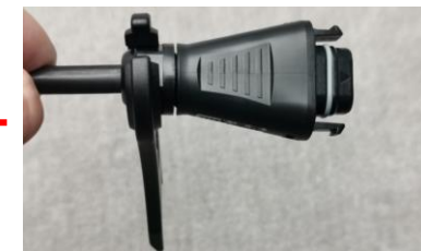
Tighten the waterproof cap with branch line breaking wrench
